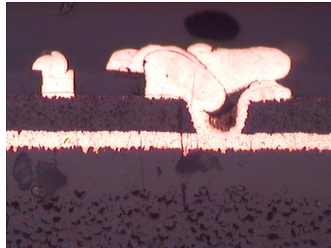
Poor additive control
